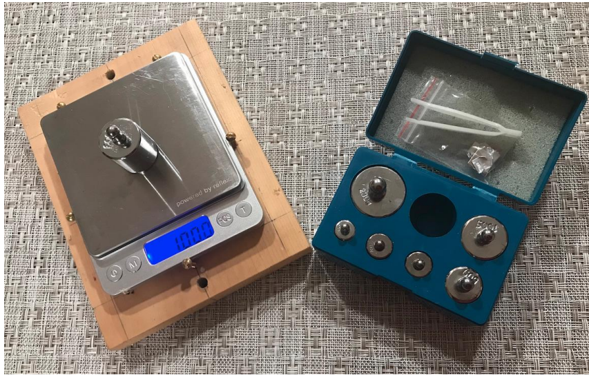
Figure A1: Scale undergoing calibration check inside at 68 F.
