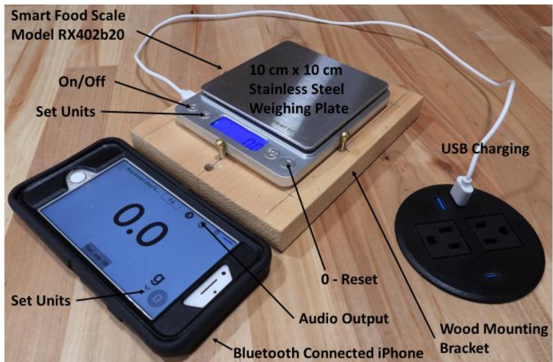
Figure 1: Scale used for avian weight measurements, Bluetooth connected to an iPhone, and being charged through its USB port.
